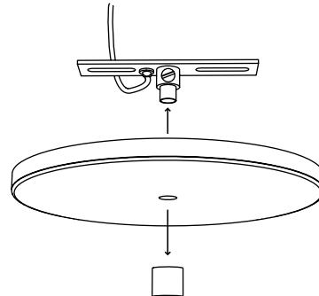
**3** Feed the cord through all pieces into the canopy, as shown in below figure.
